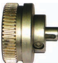
Lower O.S. without Spring (Dampening Roller Bearing Housing for Speed Master 72V & 102V/z)
